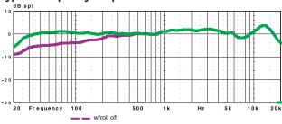
The frequency response curve shown (measuring tolerance at ±3dB) and polar pattern correspond to typical production run specifications for this microphone.
